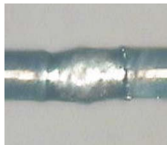
Guide Wire Welding
